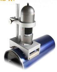
The MS-W1 is a special stand to be used for rolling forward or backward on flat and cylindrical surfaces. A great solution for checking flat objects such as paintings.
